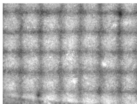
**The image of the mesh taken by using the P43 phosphor screen**
