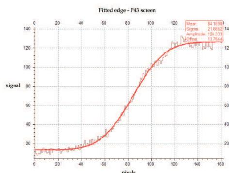
**The edge fitted by a distribution function, image taken using P43 screen**
