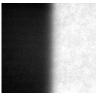
**The image of the edge taken by using the P43 screen**
