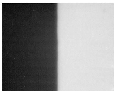
**The image of the edge taken by using the thin YAG:Ce screen**
