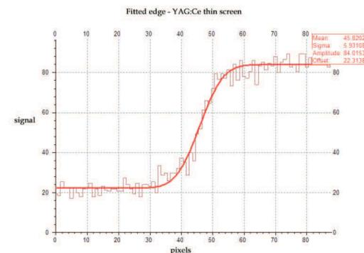
**The edge fitted by a distribution function, image taken using YAG:Ce screen**
